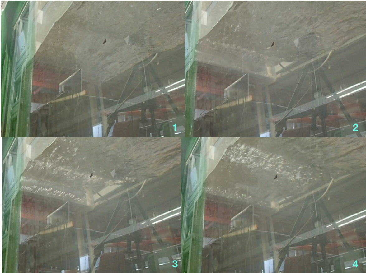
Figure 4.9: Bottom view of wave profile and air involvement changing process under r_A 60s
