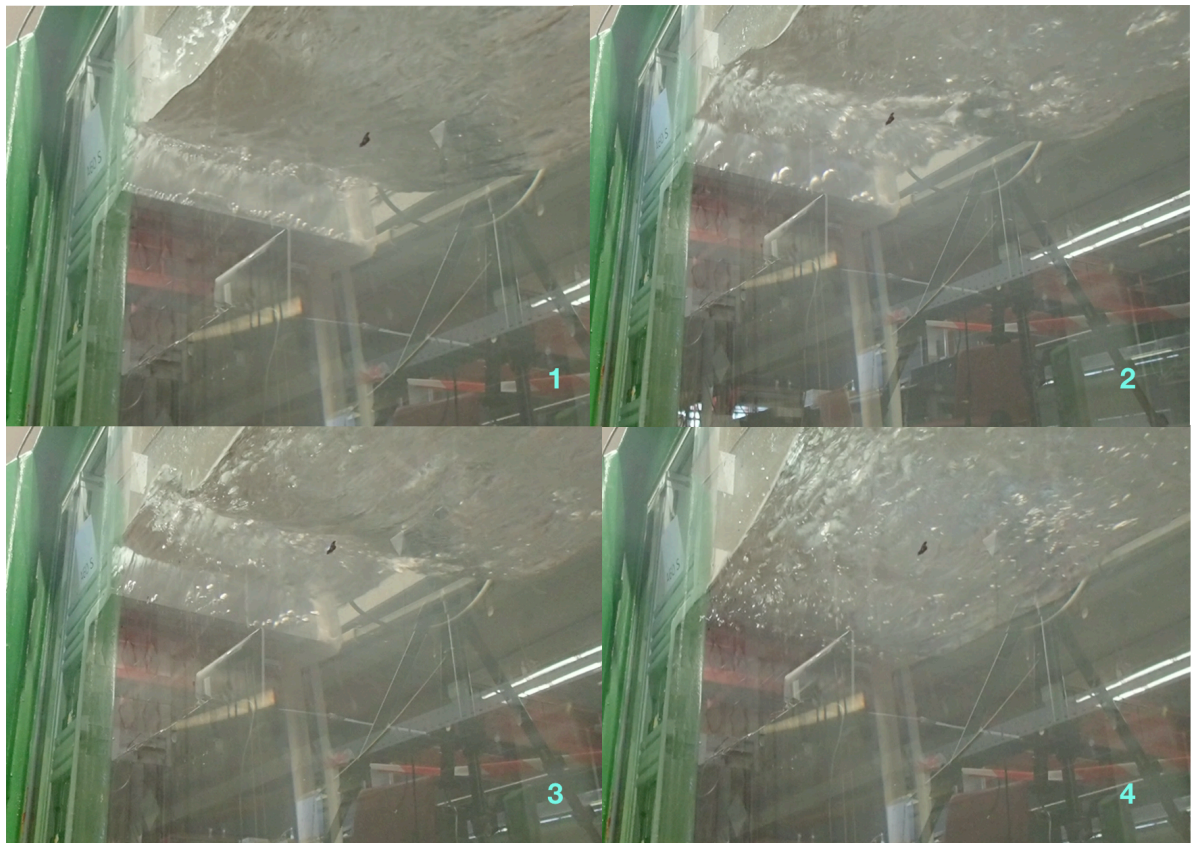
Figure 4.12: Normal pressure measurement situation under irregular waves A60s (bottom view)
