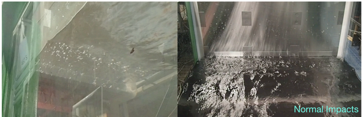
Figure 4.11: Normal pressure measurement situation under irregular waves A60s
