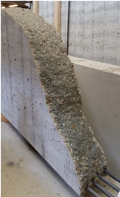
Fig. 6.10: Crack surface of the beam in reality (left) and in MATLAB presented as a point cloud with the 5 sections along the y - axis (right)
