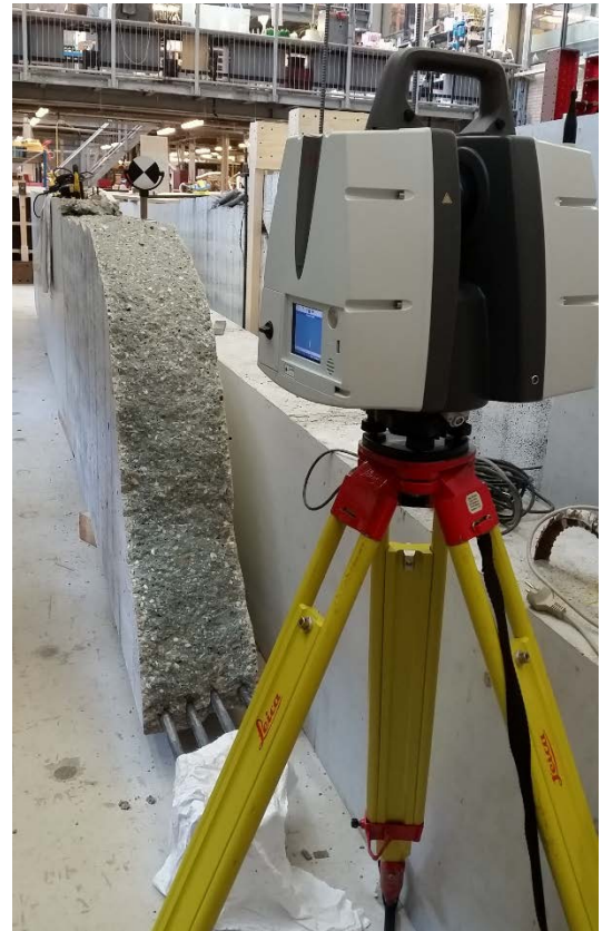
Fig. 4.6: The laser scan station and the beam
