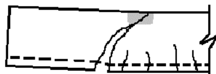
Fig. 1.2: Shear compression failure
