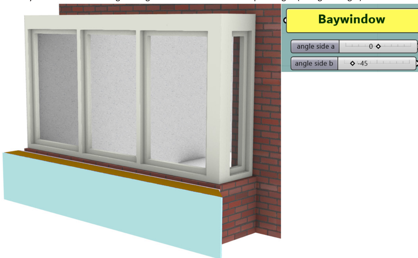
Image 106: Showing the angle on the side of the bay-window panel and its method specific input (Source: Own image)
