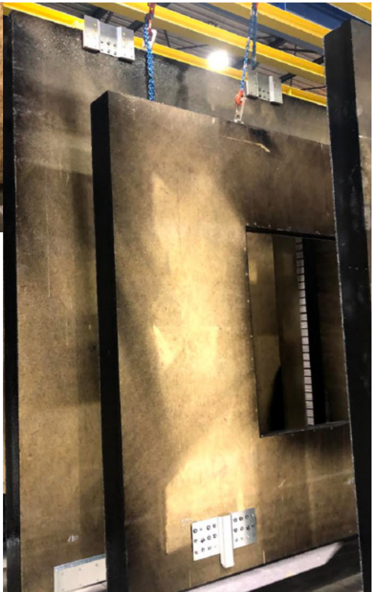
Image 15: Mounting brackets used on prefab panels by RC-panels (Source: R. Nuñez Larios)
