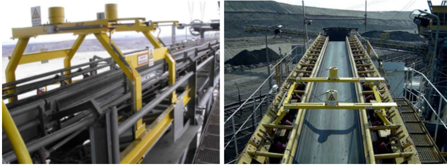
Fig. 7 Radiometric sensor measurement device
