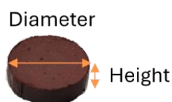
Figure 25. Measurement locations of the cylindrical green-body pellet.
