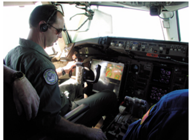
Assessment pilot Kiggins of the US Air Force uses the synthetic vision system developed at TU Delft to fly the approach to runway 7. For the test flights, a special LCD display was fitted in front of the existing pilot instruments, with the control display on the left, and the navigation display on the right. At the moment the picture was taken, with the aircraft 6 miles away from the runway, the pilot selects a new navigation display scale on the control panel to obtain a view with more detail.
