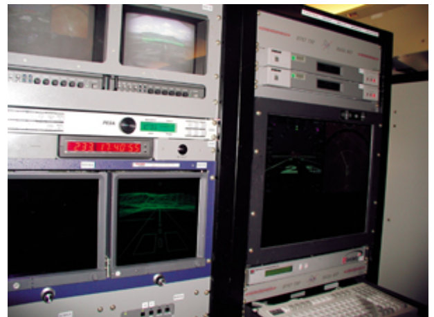
The Boeing 757 ARIES is filled with instruments, computers, and researchers monitoring the systems and pilots' actions through dozens of displays. Flights often last four and a half hours, during which time ten to eleven approaches will be flown.
