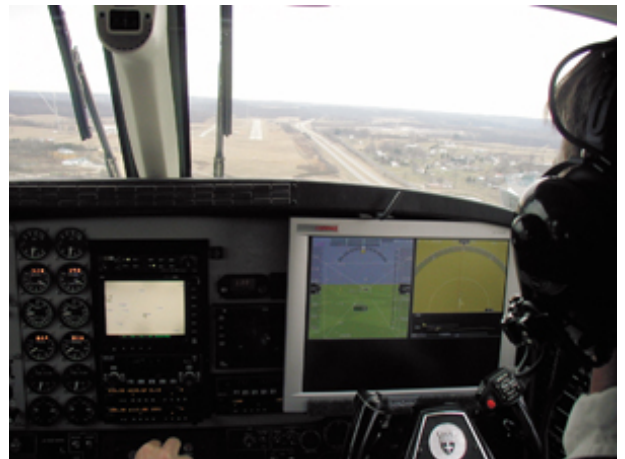
The DELPHINS synthetic vision system can also be used in smaller aircraft. In the context of the NASA Small Aircraft Transportation System (SATS) research program, a King Air research aircraft from Ohio University was equipped with the DELPHINS system. The picture on the right shows the synthetic vision display in use during an approach into the airport of Athens, Ohio.
