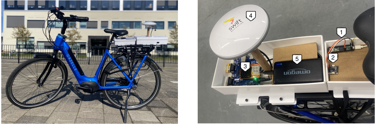
Figure 2.4: Experimental bicycle setup used for data acquisition. The left image shows the data collection systems housed and mounted on the bicycle's rear rack. The right image provides a more detailed view of the data acquisition systems. The numbered labels indicate the individual components: 1) Teensy 4.1 microcontroller, 2) SparkFun MPU-9250 Breakout IMU, 3) evaluation board, 4) GNSS antenna, and 5) external power supply. The left subfigure illustrates the housing of the data acquisition systems and their attachment to the rear rack of the bicycle. Notably, the GNSS antenna is mounted on a wooden to minimize potential GNSS signal disruptions.
