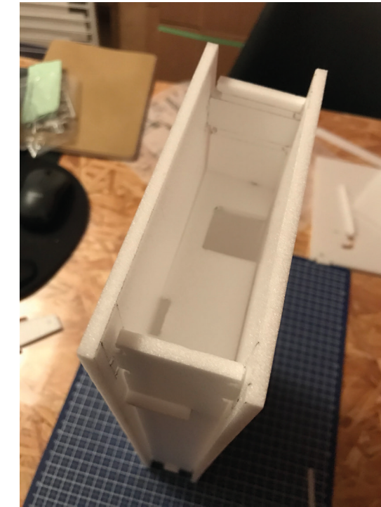
CNC-milled connection; no connectors needed
