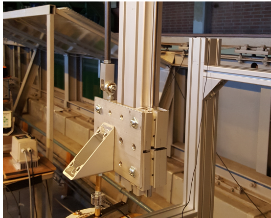
Figure 3.4: Rail system, on vertical beam with grooves, as part of motion system setup
