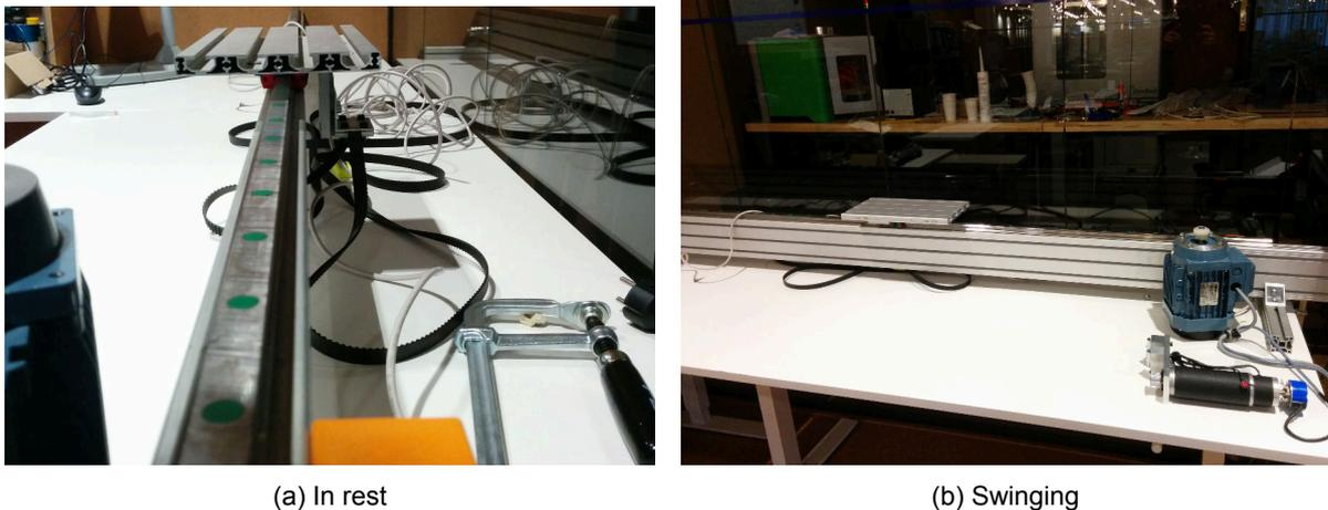
Figure 5.8: A swing for rotational testing of the IMU Euler angle results. In (a) the swing is in rest, in (b) the IMU is swinging.
