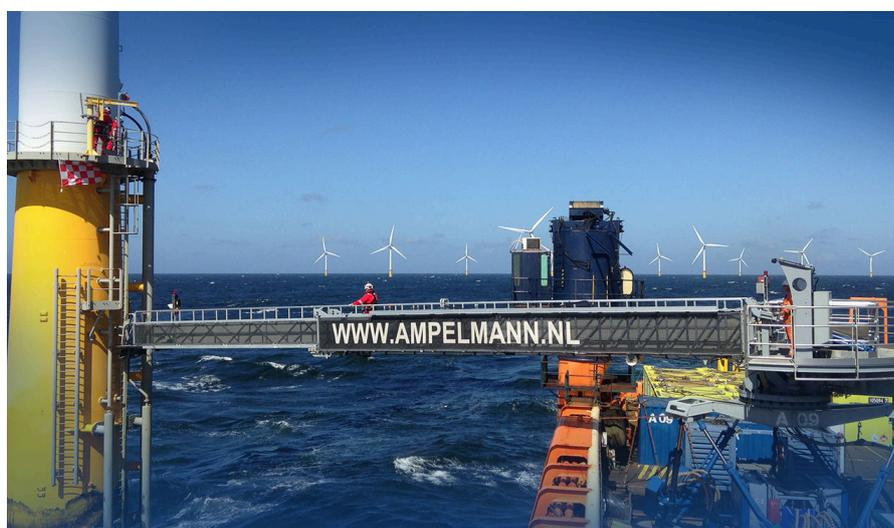
Figure 1.1: The Ampelmann system used to safely transfer people from a vessel to a offshore windmill.
