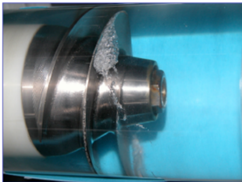
(a) Attached leading edge cavitation
