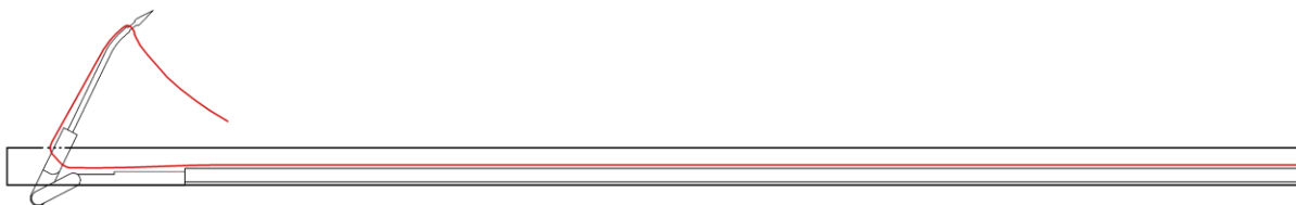
Figure 14: Concept A, the flow of the thread through the shaft.
