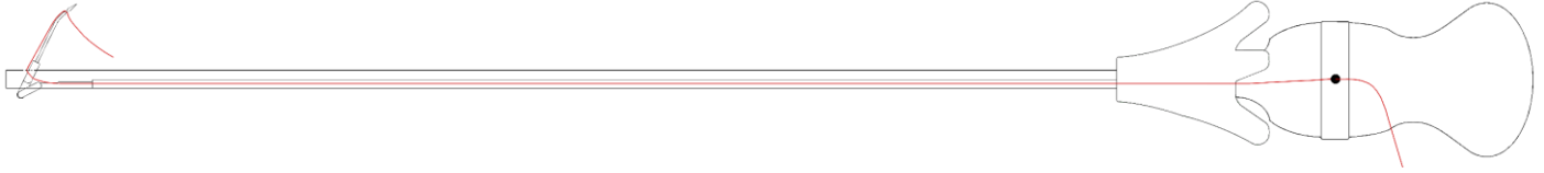
Figure 21: Flow of the thread through the instrument.
