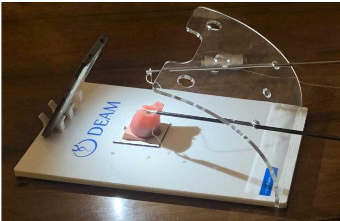
Figure 57: Lapro-trainer from DEAM with a silicon vaginal cuff model, the instruments for the Hornet method and a phone for extra lighting.
