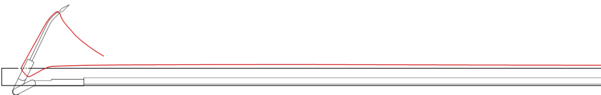
Figure 15: Concept B, the flow of the thread along the outside of the shaft.
