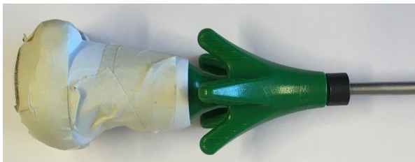
Figure 40: Model of the handle shape to test the usability of the Roticulator (the green component).
