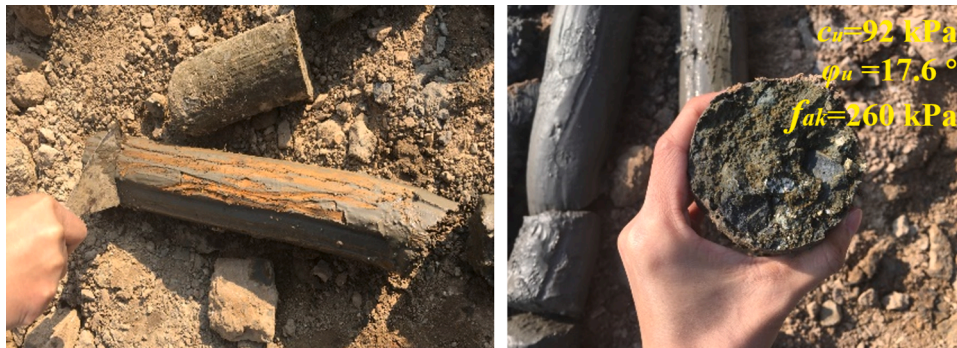
Fig. 7. Very stiff soils called Yangtze River delta clays (Images by Dagang waterworks project team).
