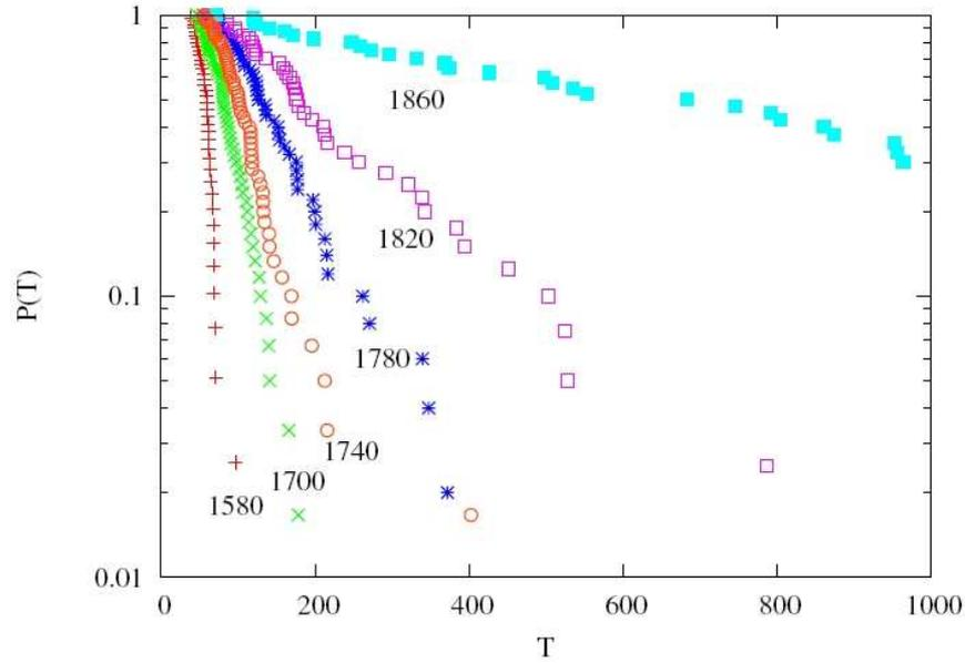
Figure 2.7: Probability  $P(T)$  of the life time of a puff to exceed  $T$ . From: Willis and Kerswell (2007a)
