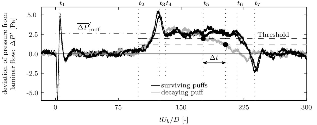
Figure 4.2: Three instantaneous time series of pressure data at  $Re = 1822$ , measured by  $PT_1$  showing two surviving and one decaying puff. The dashed black line is the threshold level ( $T_1$ ) used to determine the location of decay, the second (dashed grey line) threshold ( $T_2$ ) is used to determine the puff disintegration time. See text for details.
