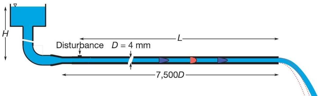
Figure 2.9: Schematic of the experiment used by Hof et al. (2006).
