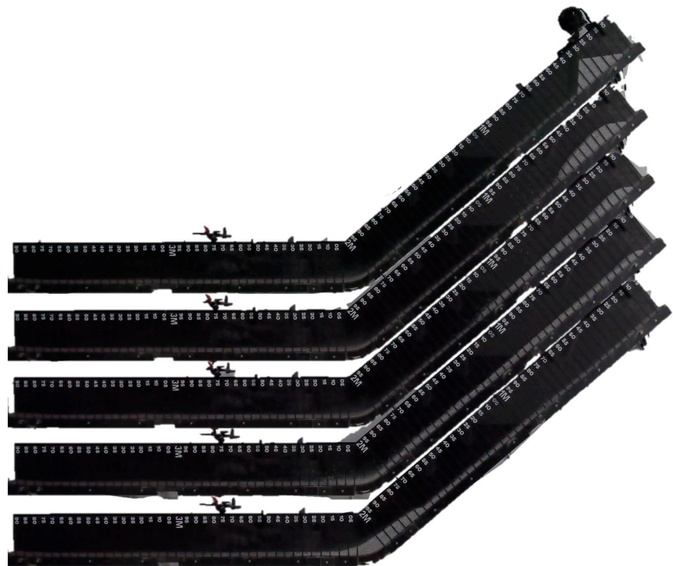
Figure 2. Material flow process in an experimental flume test at times of (in descending order) 0.258 s, 0.559 s, 0.903 s, and 2.322 s.
