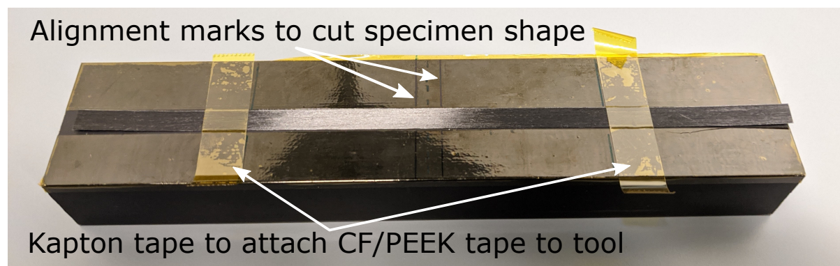
Figure 4.6: Black painted aluminum c-profile to place, align, and laser deconsolidate the specimens.
