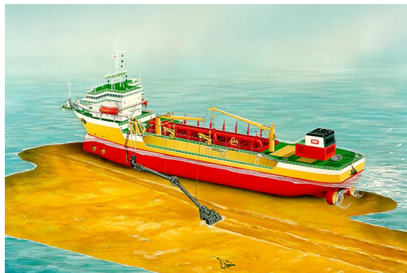
Figure 4.1. Artist impression of a trailing suction hopper dredger (Delft Center for Systems and Control, 2008).
