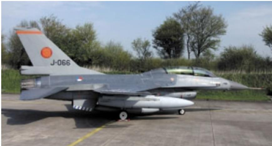
**Figure 1.3:** F-16 External 370 gallon fuel tank [106]
