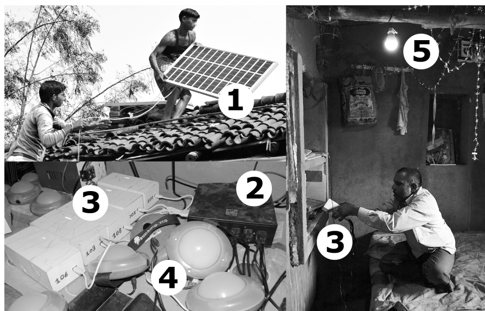
Figure 3.4: Energy Distribution Infrastructure. Note the labels: '1': Solar Panel; '2': Energy Router; '3': Power banks; '4': Solar Lantern; '5': LED Bulb.
