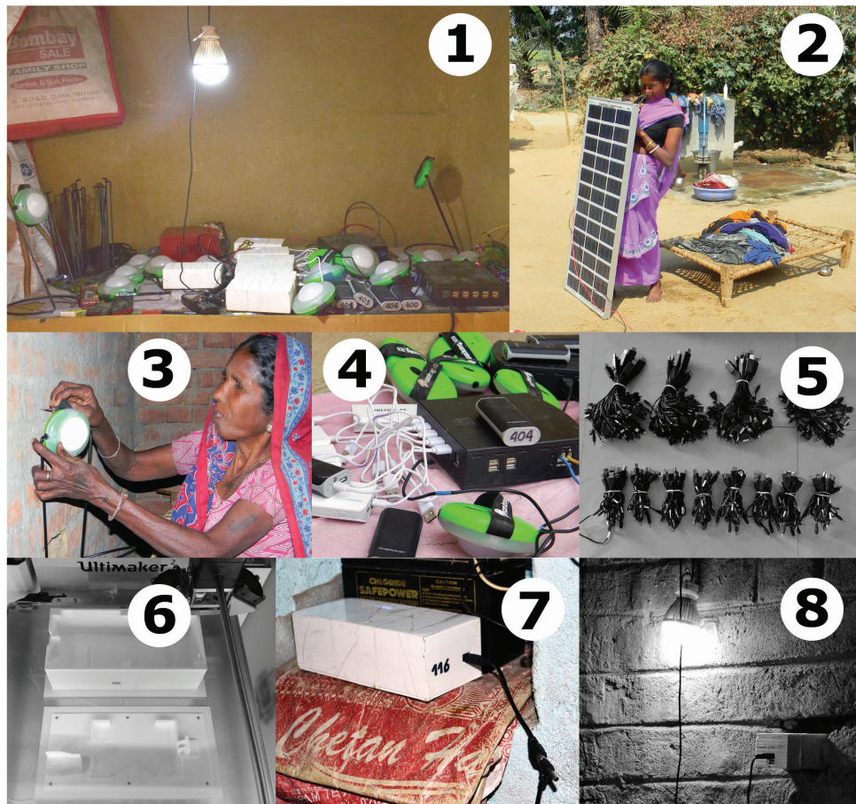
Figure 4.4: Off-Grid Energy Distribution Infrastructure. Note the labels: '1': Charging Station; '2': Solar Panel; '3': Solar Lantern; '4': Energy Router; '5': Cables; '6': 3D printed casing of the power-banks; '7': a power-bank in use; '8': a LED Bulb connected with a power-bank.
