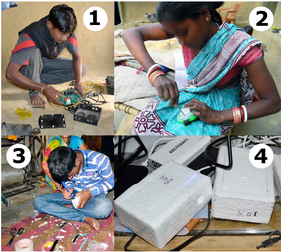
Figure 4.6: Reconfiguration of various elements of the prototype. Note the labels. '1': Soldering of a broken energy-router; '2': energy-giver repairing a solar-lantern at Manpur; '3': a family member of energy-giver at Rampur redesigning the casing of power-banks using locally available materials; and '4': redesigned cases of power-banks Rampur.
