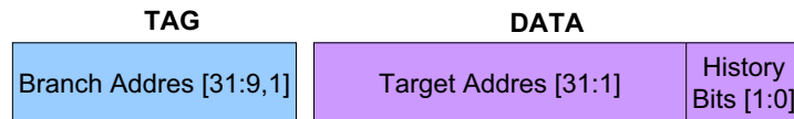
Figure 5.17: Illustration of a BTB entry in the case of a bimodal predictor (Courtesy: [64]).
