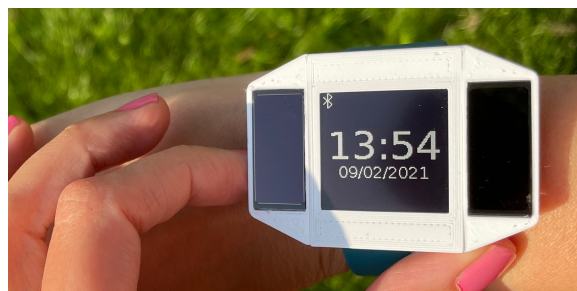
Figure 1: First battery-free open-source [1] smartwatch with FreeBie: intermittently-powered bi-directional BLE link.
