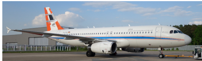
Figure D.9: Airbus A320 with HLF fin during 2018 flight tests [42].
