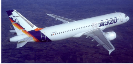
Figure D.8: Airbus A320 with HLF fin during 1998 flight tests [8].
