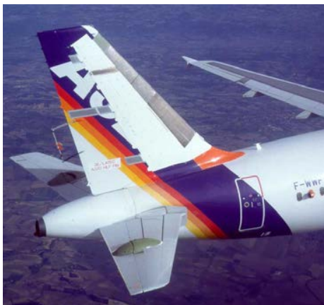
Figure D.10: Hybrid laminar flow fin during 1998 flight tests [41].
