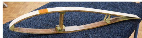
Figure 4.13: Airfoil with Delft Laminar Hump in orange 6 .
