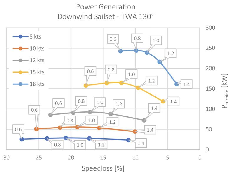
**Figure 2.16:** Regeneration study for a Panamax-sized wind-powered ship. Operating points show the propeller P/D ratio (from 0.6 to 1.4) [73].
