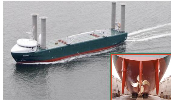
(b) E-Ship 1 with tri-rudder configuration [79].
