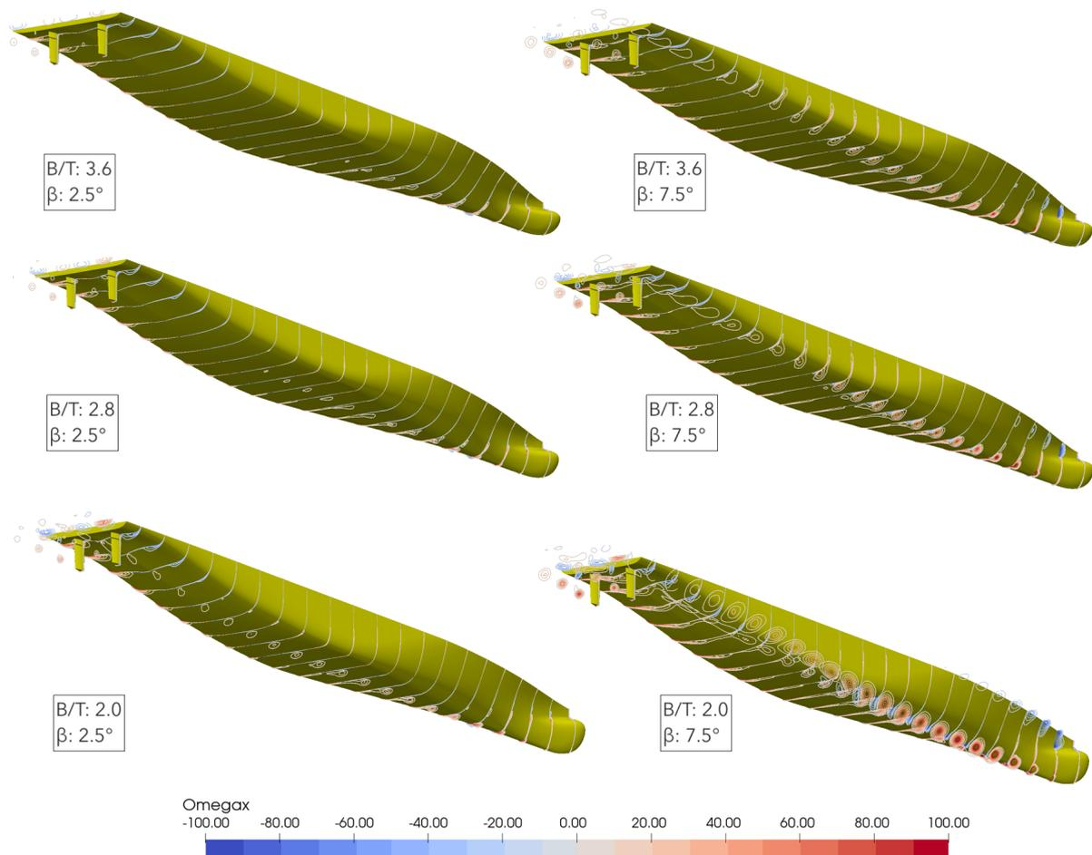
Figure 4.2: Vortex development between drift angles of 2.5° and 7.5°.
