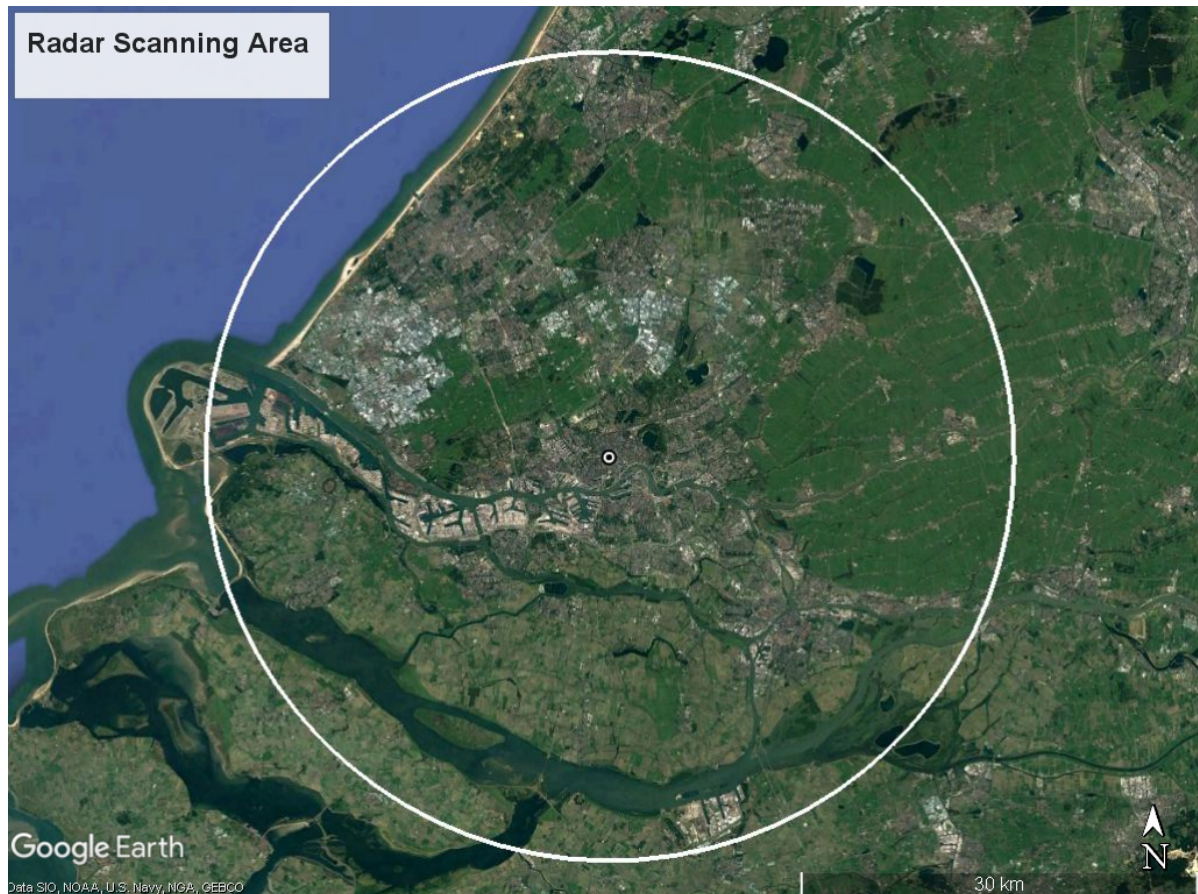
Figure 3.2: Rijnmond radar coverage area. The radius of the coverage circle is 30.48 km
