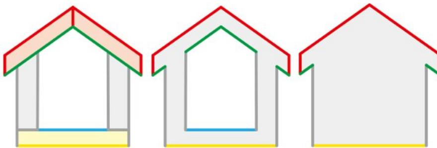
Figure 2.1: Extraction of the exterior surface of IFC solids. [[Donkers et al., 2016](#)]
