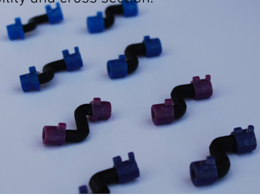
Figure 83: Variations in wall thickness, flexibility and cross section.
