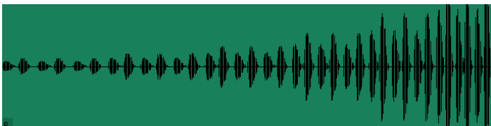
Figure 9.2.5 Eight levels of vibration intensity
