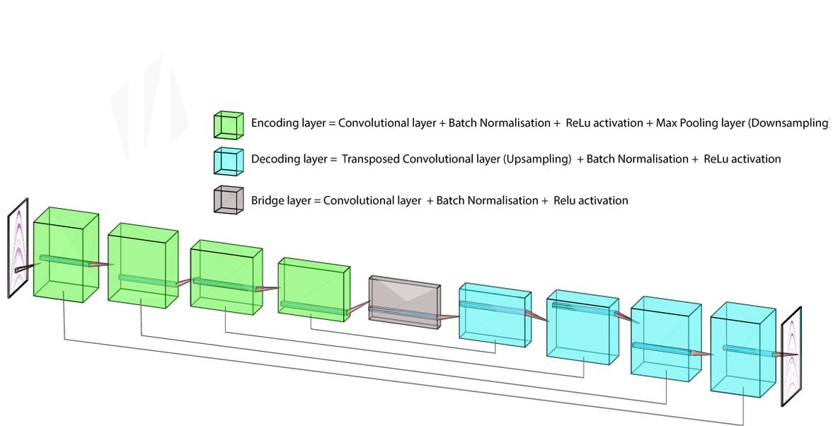
Figure 8: The architecture of the convolutional neural network, showing the encoder-decoder structure and the residual connections between each encoding and decoding block.
