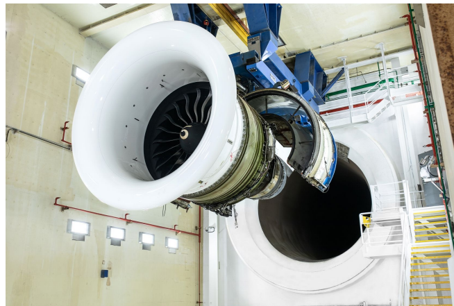
Figure 7.2: Engine equipped with bell-mouth inlet in test cell [68]
