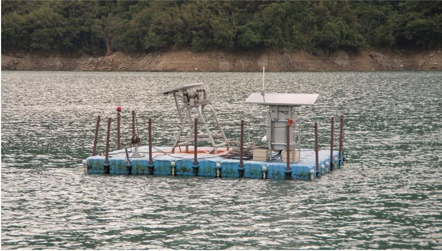
Figure 3.8: One of the floating platforms in the Shihmen Reservoir where a TDR device is placed on, November 2014.
