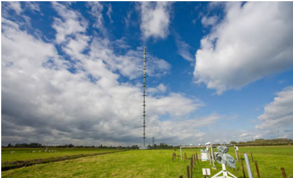
Figure 4.21: KNMI Cabauw measurement station. At the tower, meteorological conditions are measured from 0 to 213 m altitude [2].
