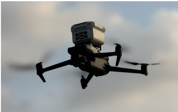
Figure 2.1: Sniffer4D Mini 2 placed on top of the DJI Mavic 3 Enterprise during the measurements in Aigaleo.
