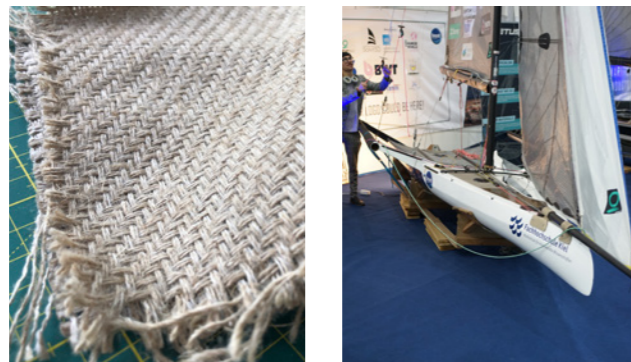
Fig. 69 right: Flax fibre weave. Right: Sailing dinghy using this construction (BOOT Düsseldorf 2025, Fachhochschule Kiel)
