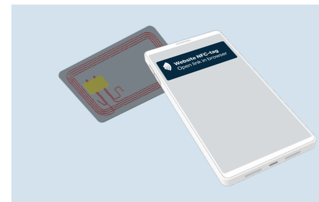
Fig. 40 NFC Chip embedded in product for easy connectivity to DPP information and automatic pop-up message on smartphone
