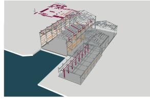
7. CLT construction for the new core
