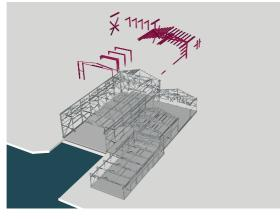
4. Removing part of construction that has been damaged due to fire
