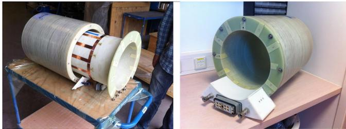
Figure 2.1: Head insert gradient coil developed at the UMC Utrecht
