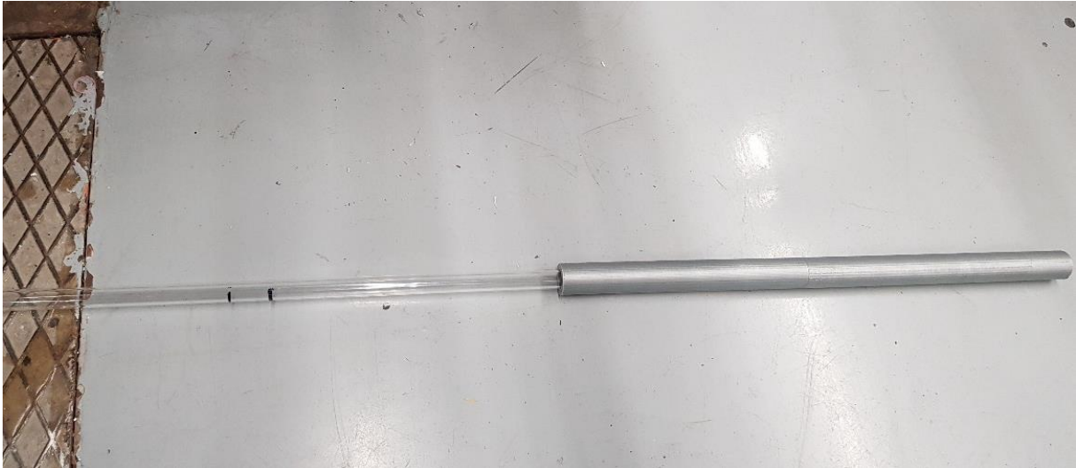
Figure 3.17: Acrylic tube inside a bigger 3D printed tube.
