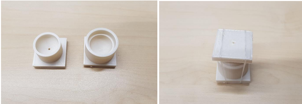
Figure 3.19: Male mould (on the left) and female mould (on the right). Figure 3.20: Moulds clamped with two elastics.
