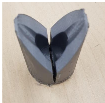
Figure 3.14: Sabot configuration inside the barrel.
