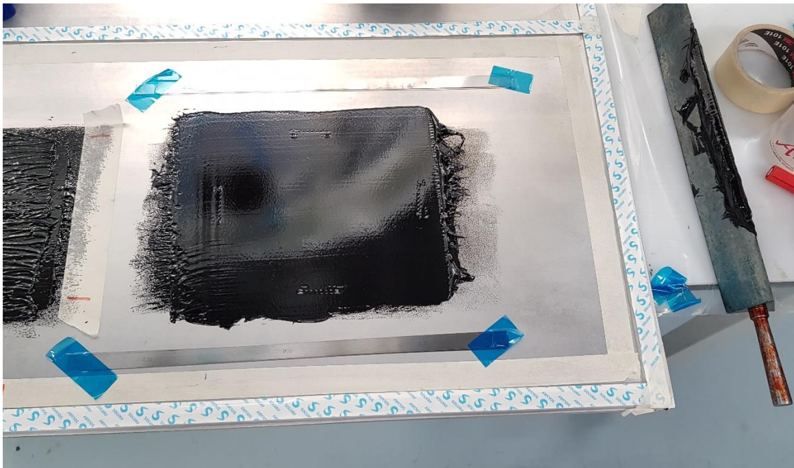
Figure 3.27: measurement points on smoothed gelcoat that is between two metal strips with the triangular tool on the right side.
