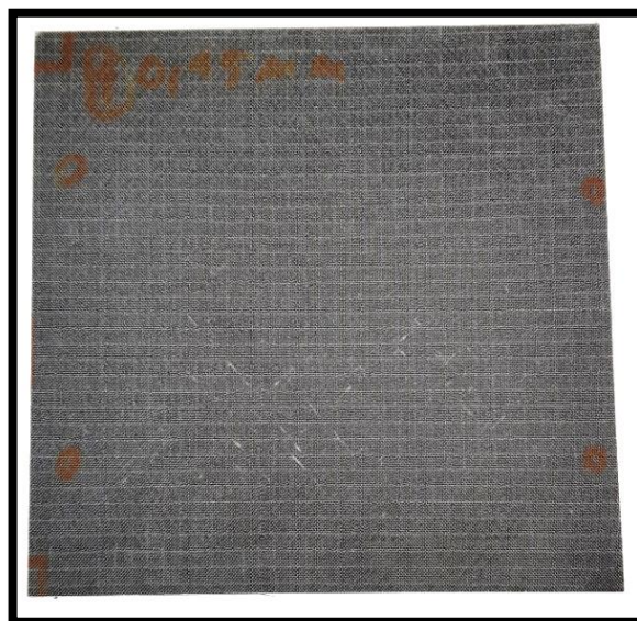
Figure 4.9: Sample 4 of CG 0.35 mm containing dry spots.
