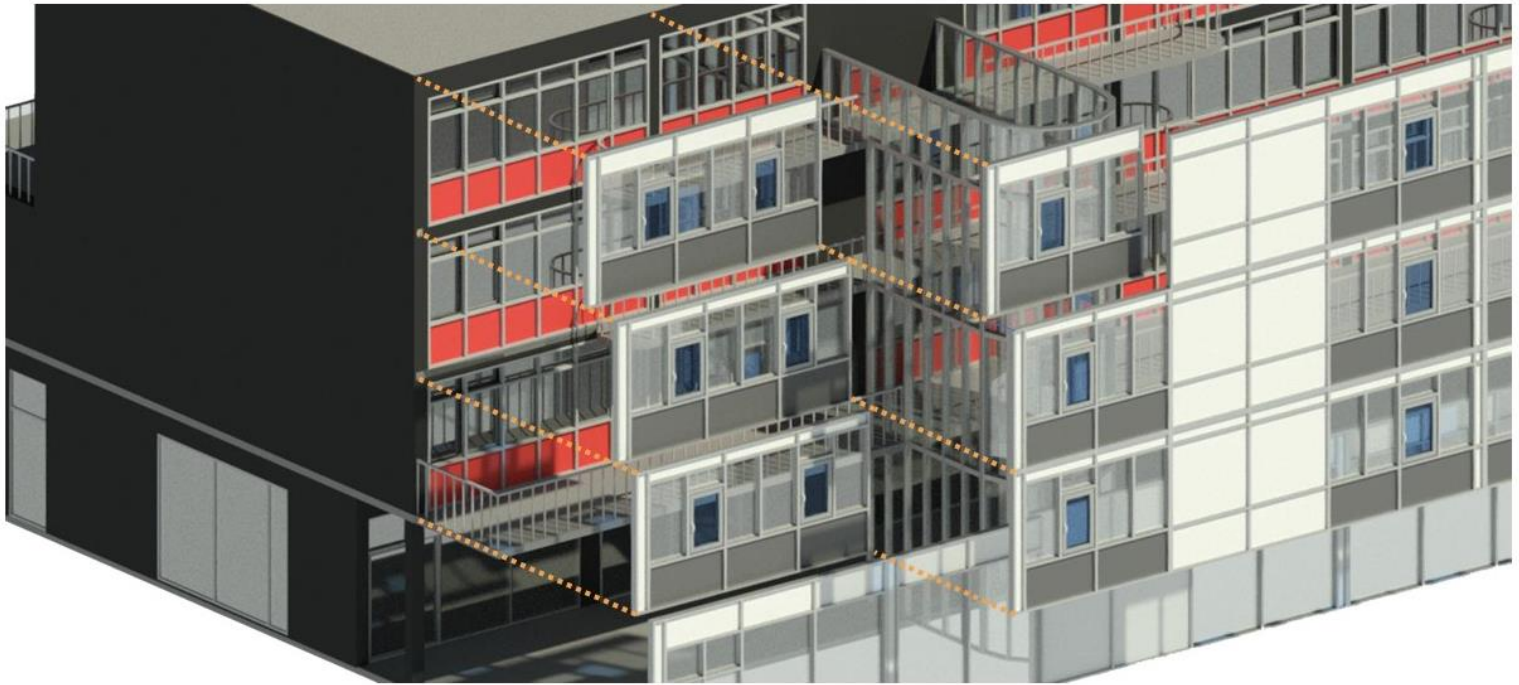
Figure 54: Schematic impression of the assembly process of the façade units on the support brackets attached to the existing structure.
