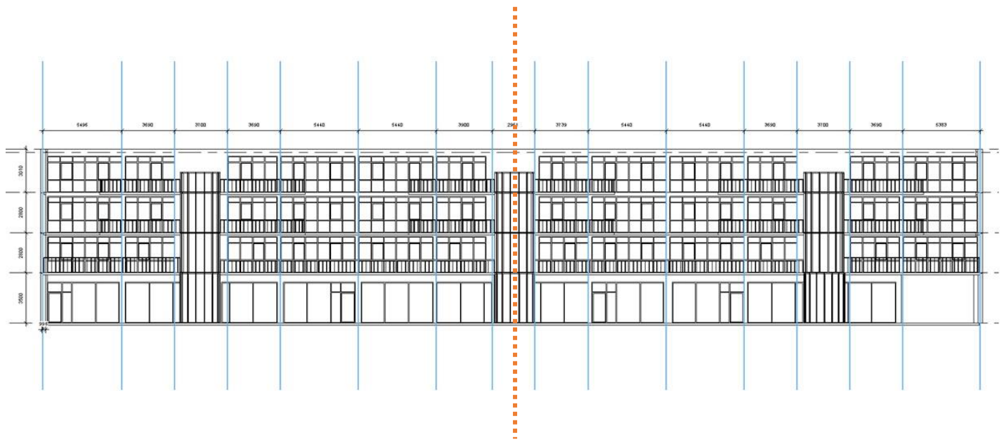
Figure 51: The grid of the façade division for the sizing of the units and the mirroring line.
