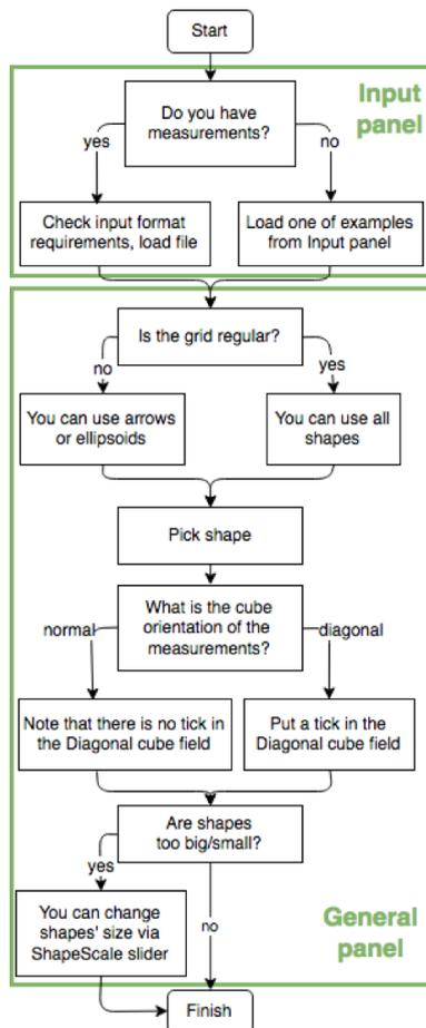
Figure 6.4: Workflow of interaction with the. First the user is supposed to upload his/her own measurements or one of the provided examples, then select and adjust adjust shapes in order to show the light properties variations in the best way.
