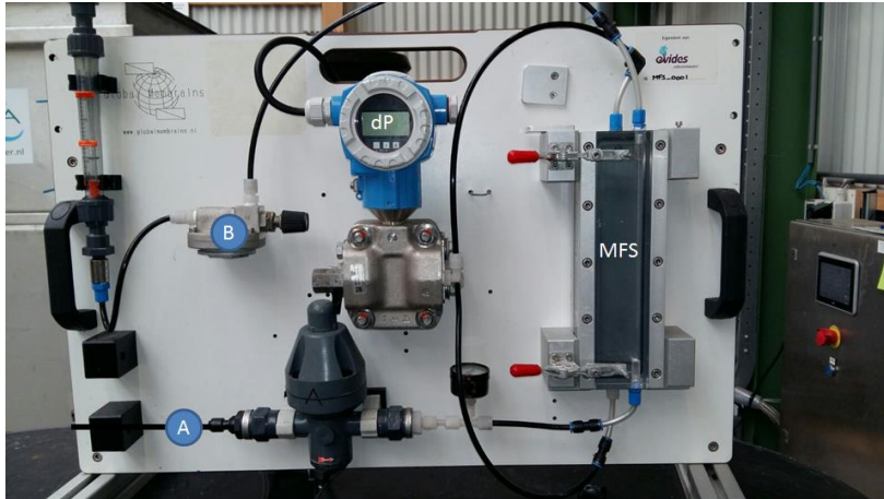
Figure 5-1. Installation for operation of the MFS. The feed flow enters the MFS scheme at (A) and is regulated with a flow controller at point (B). The pressure drop over the MFS is measured with the differential pressure transmitter (dP) (Endress+Hauser Deltabar S: PMD70).
