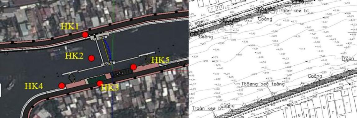
Figure 8: Boring locations and bed profile
