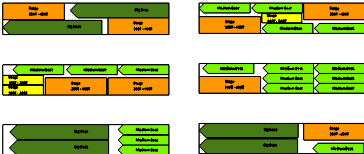
Figure 11: The 6 possible combinations for the lock, the 300T-400T barges are interchangeable with 500T-700T barges
