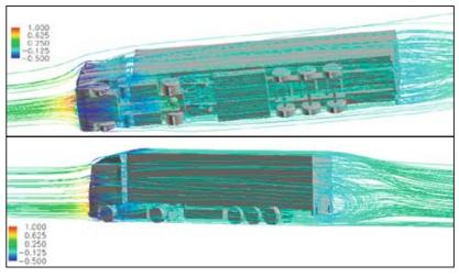
Gandert van Raemdonck aims to gain greater insights into how airflows stream along a truck when it is driving. He uses *computational fluid dynamics* to model the airflows of the truck. The computer program allows him to turn the truck in such a way that he can study it from all sides.
