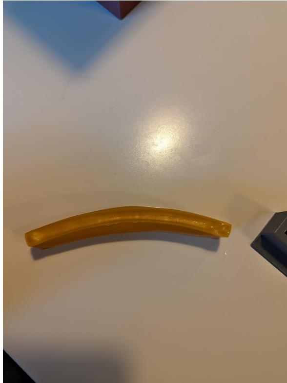
Figure 3.26: 0% infill sample printed at a layer height of 0.1mm after the programming step. Notice the concave top layers of the sample and the bulging sided
