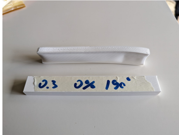
Figure 3.28: 0% infill sample printed at 0.3mm layer height after the recovery step. The sample is exhibiting swelling and bulging of the sides. the short end have become concave
