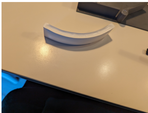
Figure 3.27: 0% infill sample printed at a layer height of 0.1mm after the programming step. This sample also has concave top layers and out of plane curving ends
