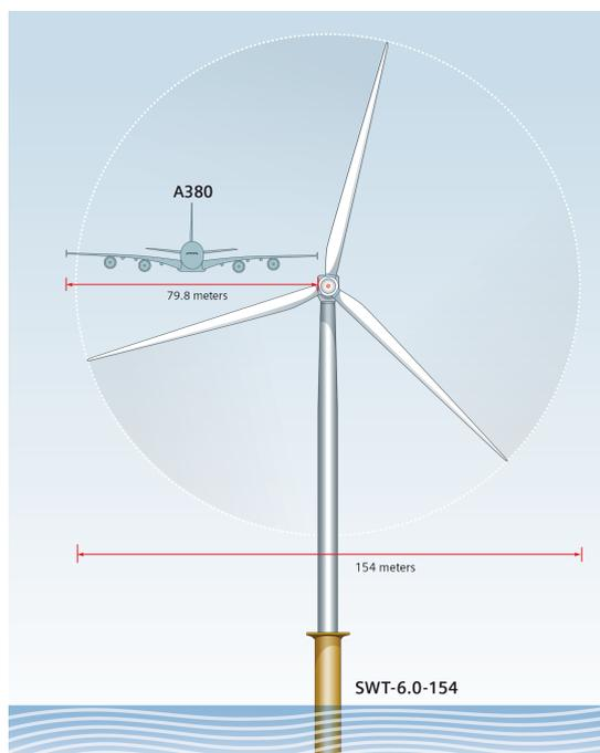
**Figure 7.1:** Illustration of the Siemens SWT-6.0-154 reference wind turbine. [7, p. 7]
