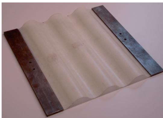
*Figure 9.2: Corrugated composite skin test specimen. [11, p. 119]*
