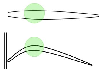
Figure 3.9: Placement of the porometer on the leaf, in top view (top) and side view (bottom).
