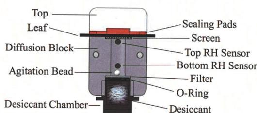
Figure 3.8: Sensor head of the Decagon Leaf Porometer SC-1. (picture from the Decagon Leaf porometer Operator's manual)
