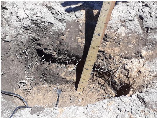
Figure 3.4: Installation of the soil moisture sensors. Photo by author.
