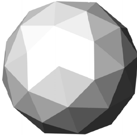
Figure C.3: The resulting icosphere with the subdivision shown in Figure C.2.
