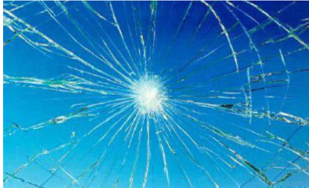
Figure 13.3: Breaking of a laminated glass pane; the glass remains together.
