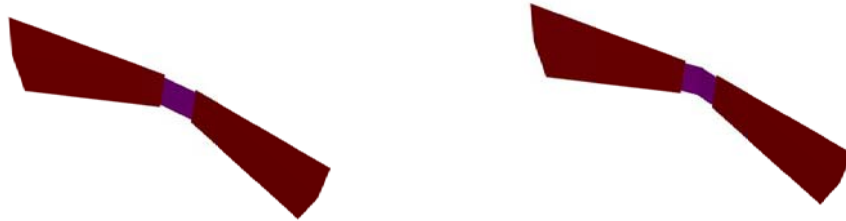
Figure 4.15: The shape of the joint in the model (exaggerated ratios!); left: the planar version; right: the 'kinked' version as proposed in Chapter 4.
