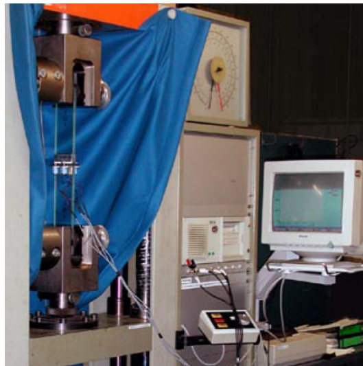
Figure 2.9: One of the tensile tests on the adhesive joints, from (Blandini & Sobek 2005).
