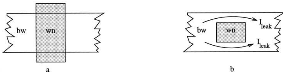
Figure 3.30: (a) WN intersects BW completely (b) WN paled within BW, according to the design rules for the NPN. Low-ohmic leakage paths short-circuit the resistor.
