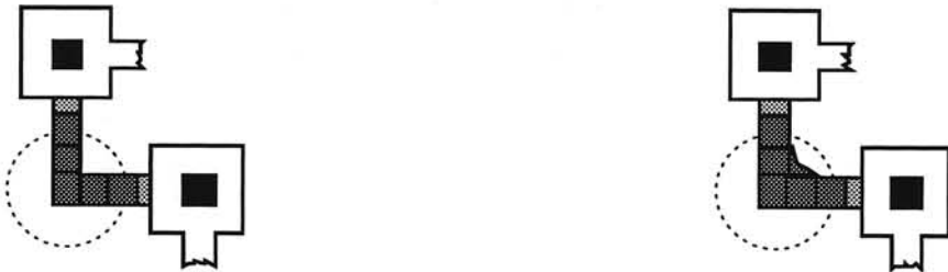
Figure 3.26: Deformation of a corner due to processing artifacts
