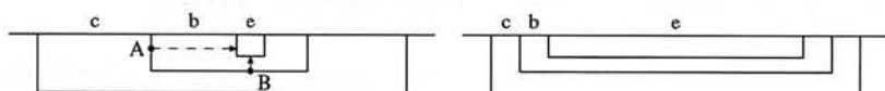
Figure 5.59: The influence of the layout on the saturation voltage. a) A transistor with a relatively tiny emitter and b) A transistor with a relatively large emitter
