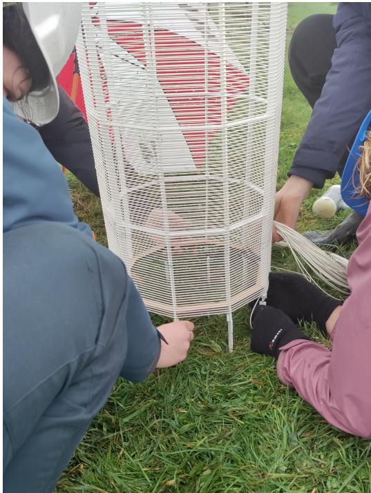
(c) The coil is glued onto the stakes.
