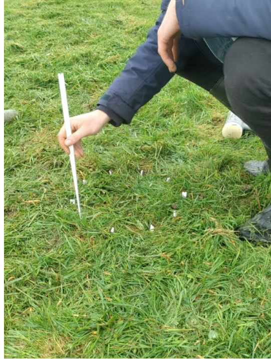
(b) The stakes being driven into the soil after using the template.
