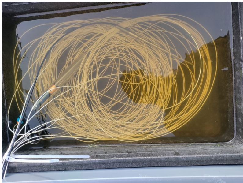
Figure 4.7: The inside of the heated calibration bath
