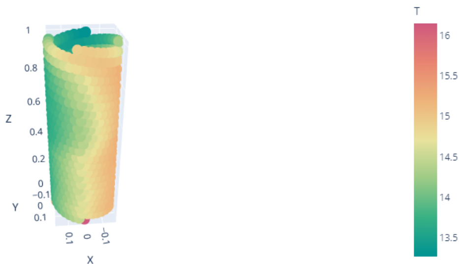
Figure 5.4: 3D plot of the horizontal ice experiment at a certain timestep. It is clearly possible to discern some variance in the horizontal direction, as is demonstrated by the distinct waterline on the coil. However, DTS accuracy and design tolerances result in a line along the length of the coil that is not exactly straight
