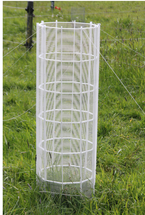
(d) The coil is tethered to the ground using 0.5mm nylon wire.
