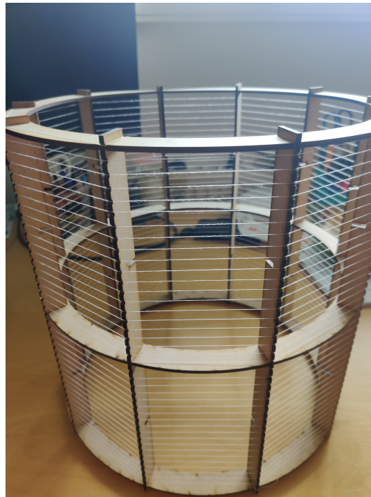
Figure 3.4: The first prototype of the initial design for the frame made out of MDF. it features circular support rings, held together by vertical struts. Thread is used to simulate the glass fiber cable.
