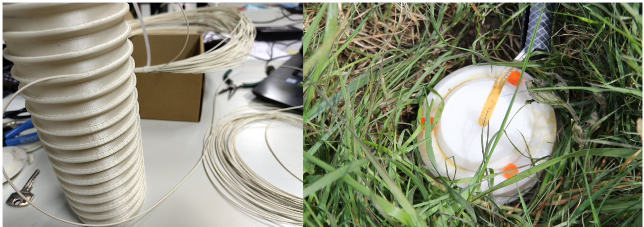
(a) Winding of the ground screw with the glass fiber cable
