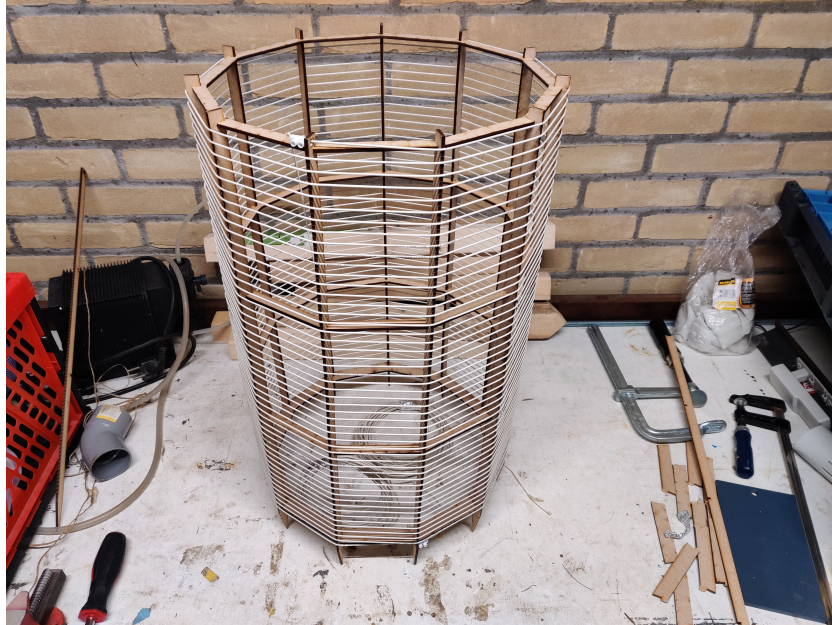
Figure 3.5: the iterated design of the coil, made out of MDF. the coil now features polygonal support rings, such that the shape of the glass fiber is followed. Additionally, the fiber is tensioned using Lester terminals at the start and end of the coil. Small stakes were included at the bottom for embedding it in the soil.
