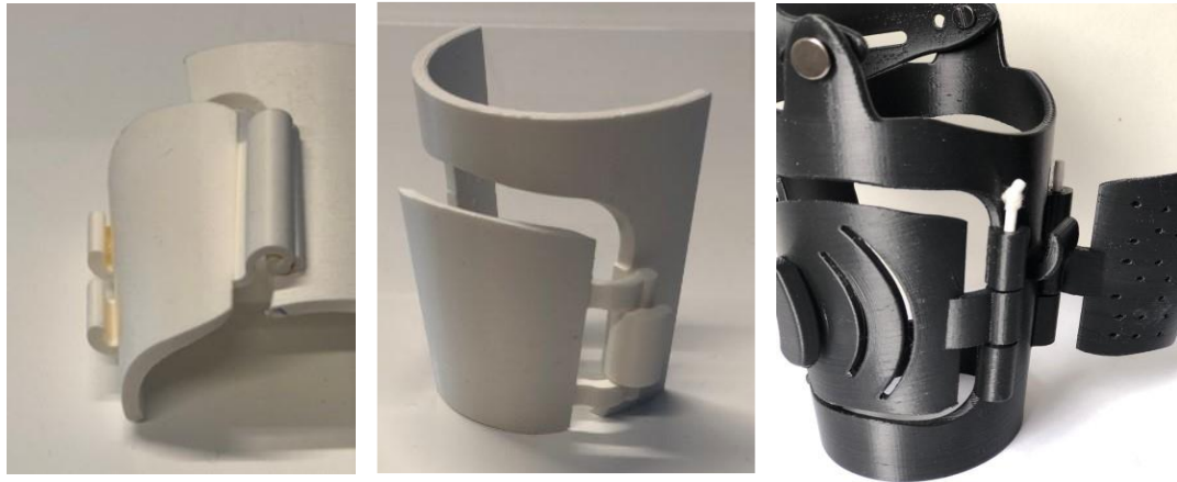
Figure 5.11. 3D printed samples of the three hinge joints. The 3-pieces hinge was the most secured design, and it was providing the widest range of volume adjustability of the wings compared to the other two designs.
