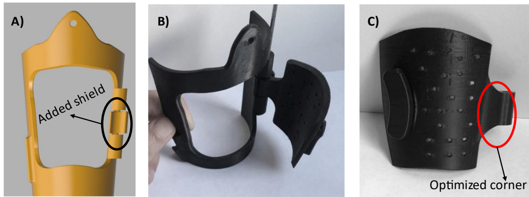
Figure 5.13. The improved version of the 3-pieces hinge. (A) Model of the hinge with the added shield that can limit the range of volume adjustability of the wings. (B) 3D printed sample of the optimized hinge with the adjustable wings assembled. (C) Optimized corner of the wings where the hinge joint is connected to the adjustable wing through a curved corner instead of a flat one that can easily break.
