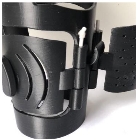
Figure 5.21. Quick built prototype of the top half of the socket for testing whether the ventilation openings would cause marks on the skin or not. The curved openings caused marks on the skin, but the 2mm holes did not. Therefore, the curved holes were adapted in the socket design as a source of ventilation.
