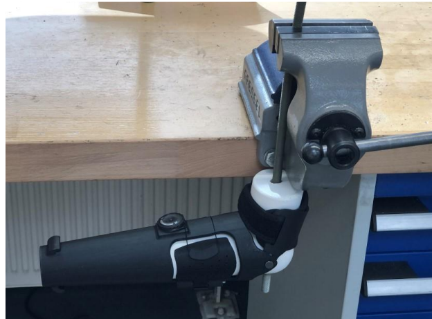
Figure 7.3. The setup of the bending test. The setup was meant to mimic the real scenario where the user would be loading the socket transversely as if the user is carrying a bag.
