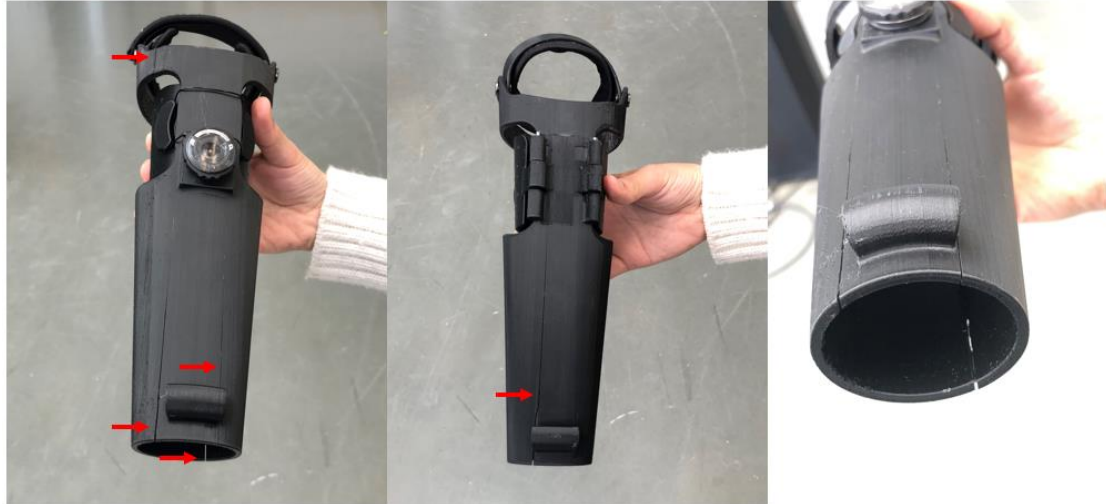
Figure 7.5. Cracks of the socket after dropping it twice from a 5m height. The socket cracked along the direction that it was printed in (printing orientation of 0° angle with respect to the printing bed) as expected. That cracking direction is the same direction where layers of filaments were adhered together. The red arrows show the locations of cracks, see the video of all the impact strength tests . The test passed the impact strength test after it was dropped from 2.4m without showing any cracks or any signs of breakage. The 5m height test was only performed to see where the cracks would develop in the socket it was hit by an object suddenly.
