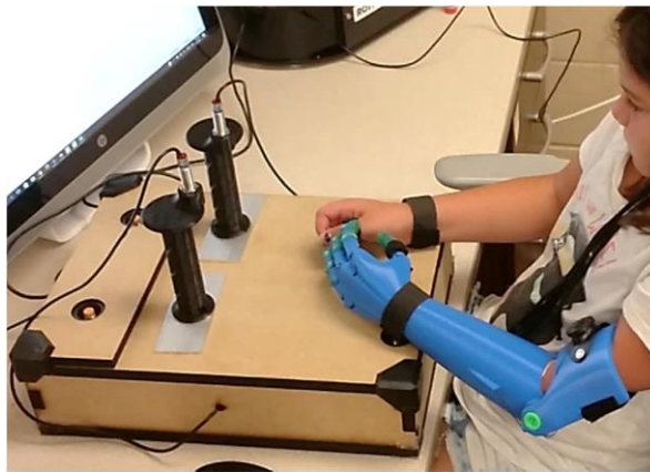
Figure 3. Transradial prosthesis with the socket integrated [28].
