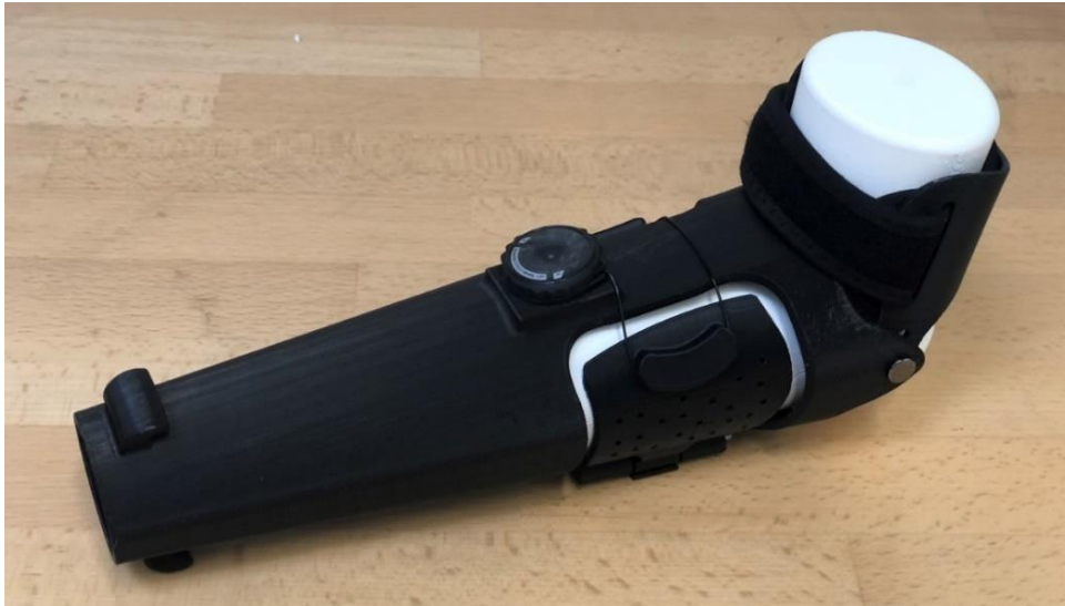
Figure 6.4. The V3D socket prototype. The socket was 3D printed from tough PLA. Then the adjustable wings were assembled to the main shell via metal threaded rod, and the lace-tensioner mechanism was snapped in the tensioner housing. After that the upper attachment was connected to the socket main shell at the elbow through flat head screws. Note that at the distal end of the socket, curved hooks were 3D printed as part of the main shell. Those hooks were modeled to only be able to perform the mechanism assessment on the prototype, and they are not part of the socket design.
