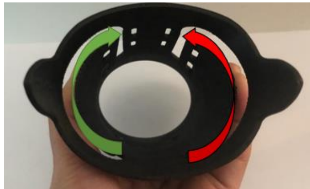
Figure 5.8. Partial (red) vs. complete (green) enclosure of the adjustable wings during tightening. Achieving secured suspension of the adjustable wings to the residual limb when it is tightened requires a complete enclosure of the wings to each of the sides of the residual limb as the green arrow shows. The printed sample does not offer that as the adjustable wings are connected to the back strip of the socket. Therefore, each wing in the current design cannot achieve a complete enclosure.
