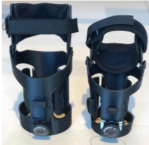
Figure 7.6. Testing sockets for the human evaluation. Two different sizes were produced to fit different participants from both genders; small and medium size sockets.
