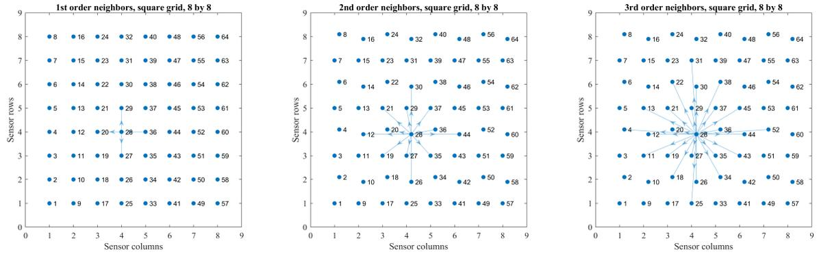
Figure 4.6: An  $8 \times 8$  array is shown with the electrodes indices denoted. Here only the connections are shown for electrodes number 28 with a square grid basis. From left to right the first, second and third order neighbor are connected. So from left to right  $\Xi^{(1)}$ ,  $\Xi^{(2)}$  and  $\Xi^{(3)}$  are shown when looking at the links originating from electrode 28.
