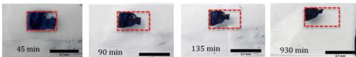
Figure 4.10: Drying of (decreased thickness on one end) 8% w/w Na-Alg barcode with change in mass and dimensions over a time period of  $\approx 24$  h. Scale bar: 2.7 mm
