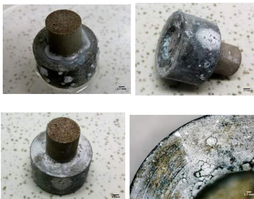
Figure C.9: Metal stamper test results showing deposits of  $\text{CaCO}_3$ . Scale bar corresponds to 2.7 mm
