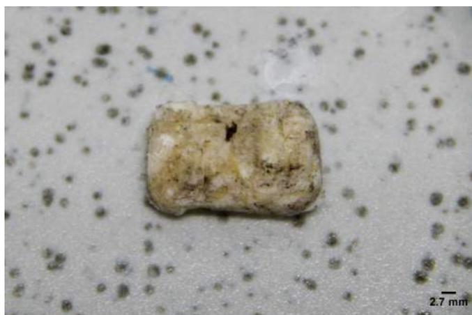
Figure C.8: Composite barcode made from lactose milk powder and Na-Alg
