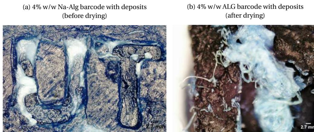
Figure 4.8: Deposits on 4% w/w hydrogel barcodes made from optimized experimental protocol. (a) Deposits on barcode before drying. (b) Deposits on barcode after drying. Scale bar: 2.7 mm
