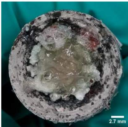
Figure 4.4: Reaction of 12% w/w Na-Alg (with HEPES) in the circular stamper after allowing the hydrogel to cure for  $\approx$  10 days
