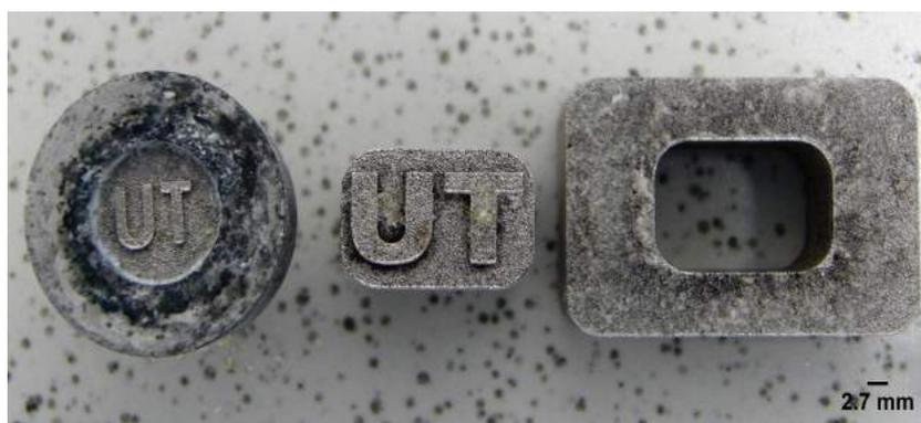
Figure 4.1: Metal stampers available that were used to cure the Na-Alg, fabricated and designed from previous work [42]. Scale bar: 2.7 mm
