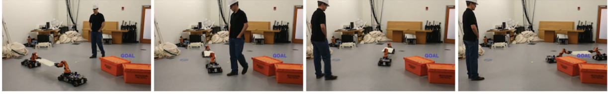
Fig. 12. Four consecutive snapshots of an avoidance maneuver where two mobile manipulators collaboratively carry a rigid object and navigate it to the goal while adjusting their formation to avoid collisions with the orange boxes and the human. Robots and human are tracked by overhead cameras. This maneuver is performed in 1 minute.
